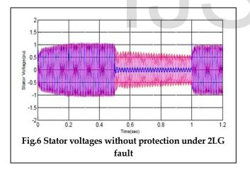
The stator (p.u) voltages without protection under the 2LG fault condition are shown in the figure 6. The fault condition is considered to occur at 0.5 seconds to 1 second, where the stator voltages are decreased from the previous constant voltage under normal condition
