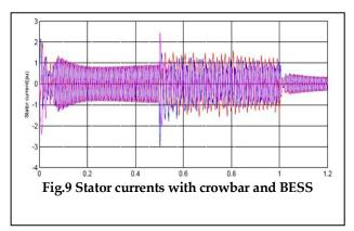
The stator currents under the fault condition with the crowbar and BESS protection are shown in the figure
