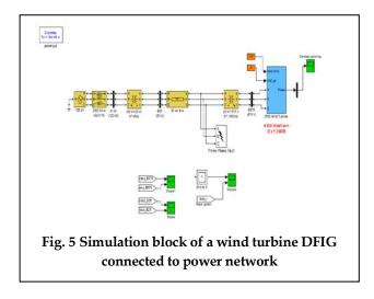
For wind speeds lower than 10 m/s the rotor is running at sub synchronous speed. At high wind speed it is running at hyper synchronous speed. The turbine mechanical power as function of turbine speed is displayed for wind speeds ranging from 5 m/s to 16.2 m/s.
