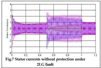
The stator currents without protection under the fault condition can be observed in the figure 7. It can be observed that under the fault condition the stator currents are increased than the previous value. These increases in currents are corresponding to the decreased stator voltages
